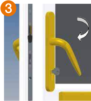
Push the handle down to retract the hook bolts and the latch. This allows the door to be opened.
