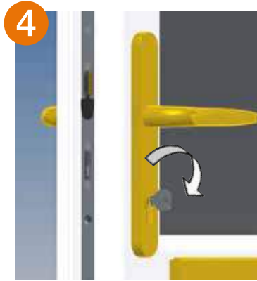
Some front-door fittings need a turn of the key to retract the latch bolt from outside. Turn the key away from the lock edge to retract the latch bolt.
